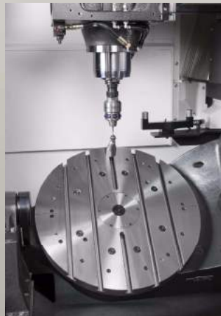
■ Worktable Center Calibration w/ Heidenhain TS740. High Precision Touch Probe & Standard Calibration Ball with Heidenhain Measurement Software can detect error value of the worktable and compensate to ensure Worktable Precision.
