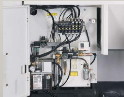
Hydraulic & Lubrication System(LU-620)
