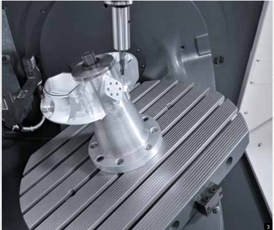
1: Flexible machining with three to five axes 2: Easy-to-see work area with an optional tool magazine 3: Simultaneous table
