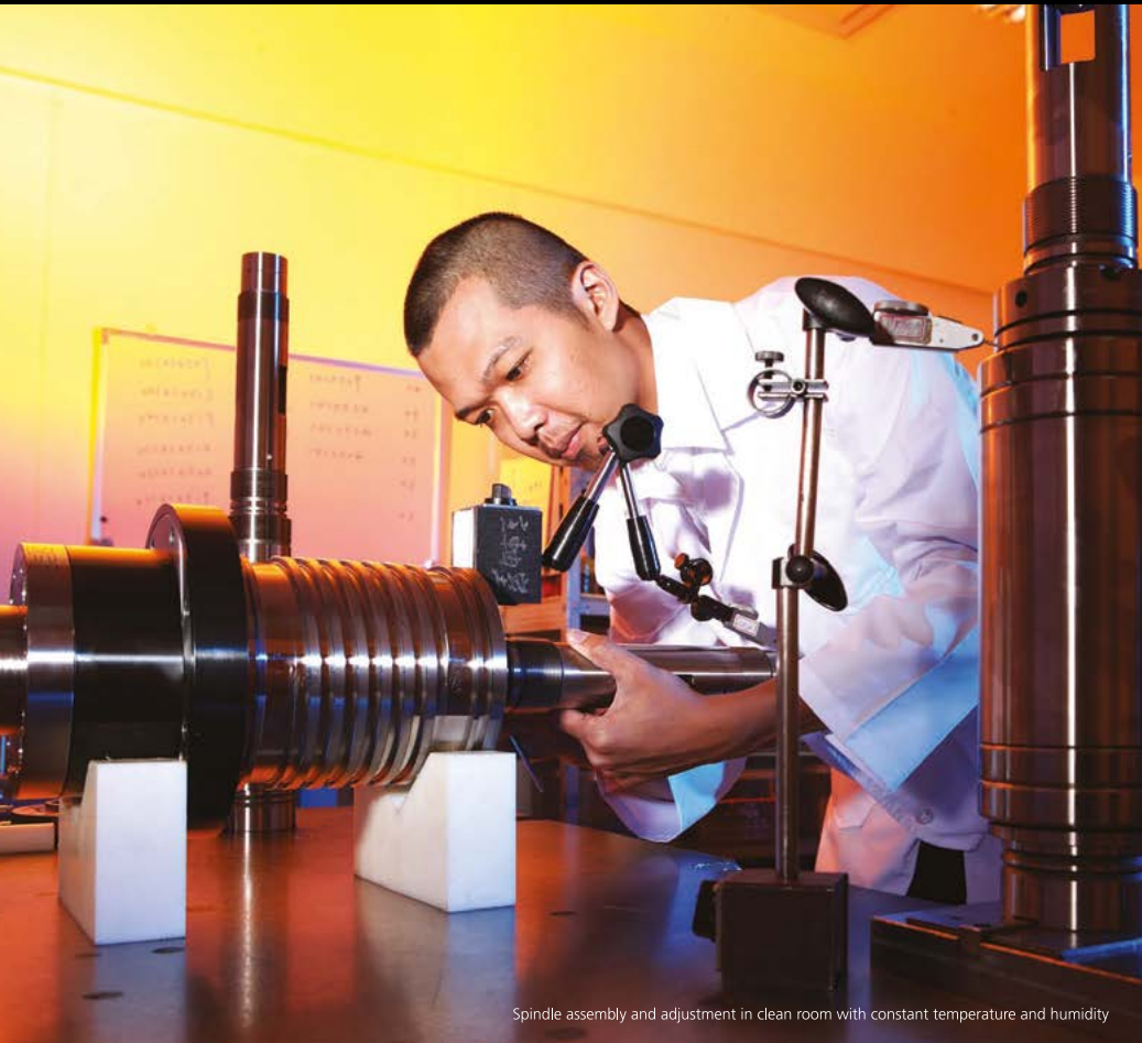
Spindle, gear box, and spindle motor balance test
