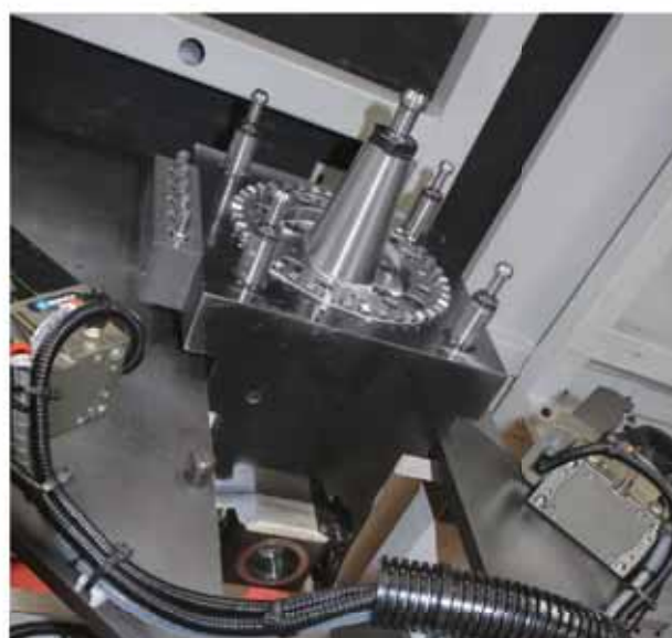
BT50 turning tool holder with 4 pull studs
