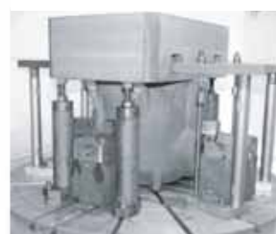
VTL1600ATC+C Hydraulic cylinder
