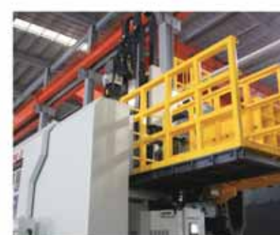
Operator's platform extension
