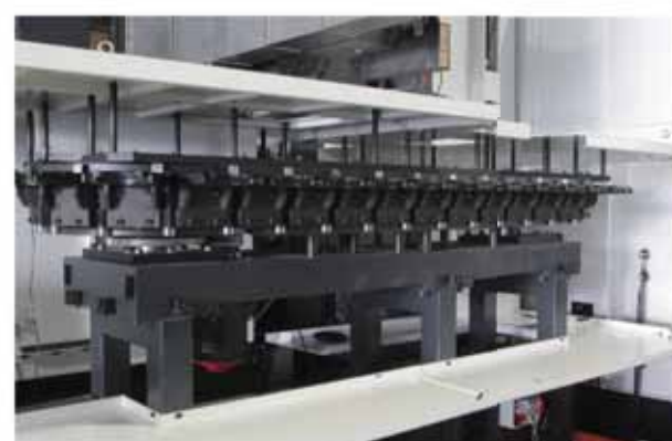
Tool magazine for 24, 32, 48, 60 tool position
