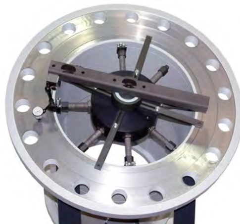
Inserting and aligning the clamping device
