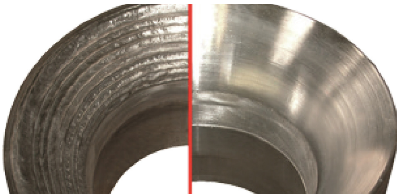
| Turning result of a funnel-shaped converging valve seat
