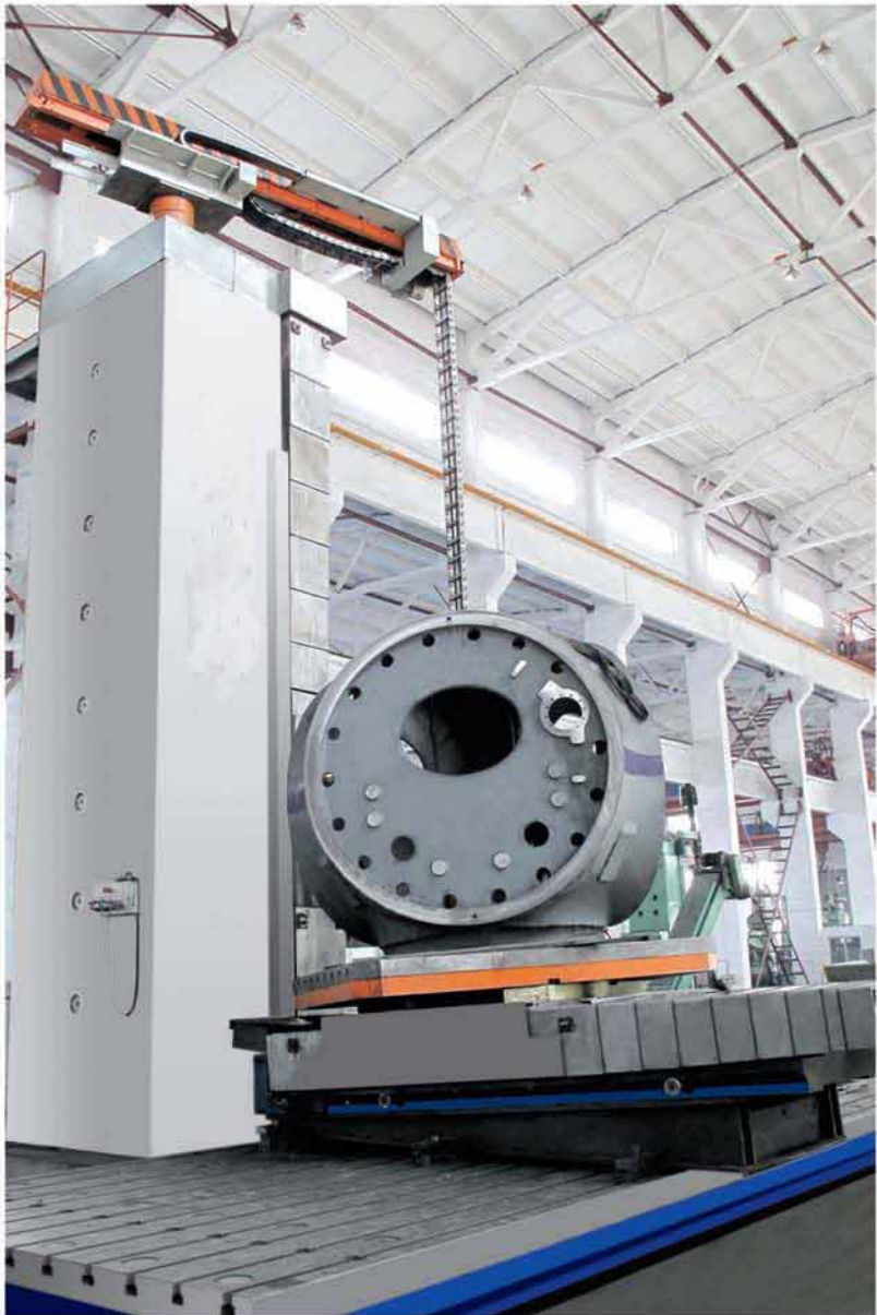
落地铣镗床正在加工风电零部件 Floor Type Milling Boring Machine while machining Parts of wind power Equipment
