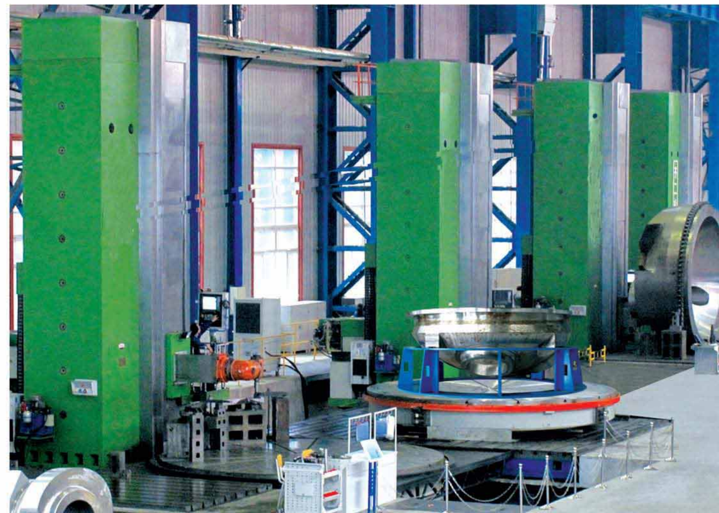
TK6920 双立柱数控落地铣镗床正在加工核电零部件 CNC Floor Type Milling and Boring Machine with Double Column while machining Parts of nuclear Power equipment
