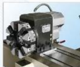
▲ Electrical system Turret
