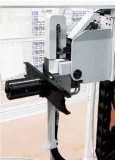
Horizontal ATC operation with a 90° head attach mounted.
