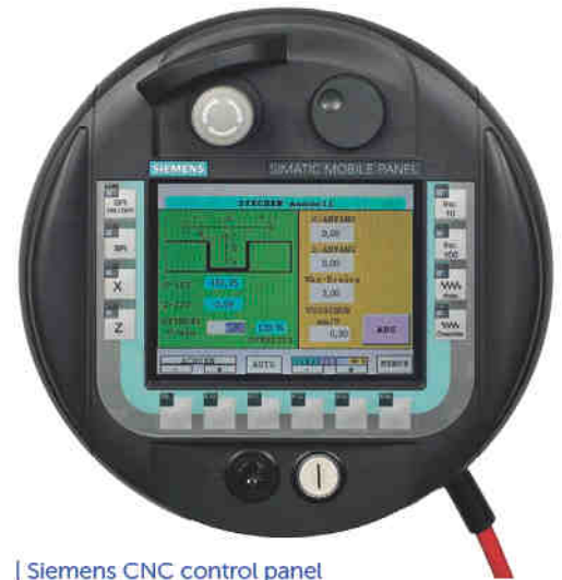
| Siemens CNC control panel
