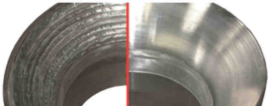
| Special type valve seat machined with a TD-2.02 NC
