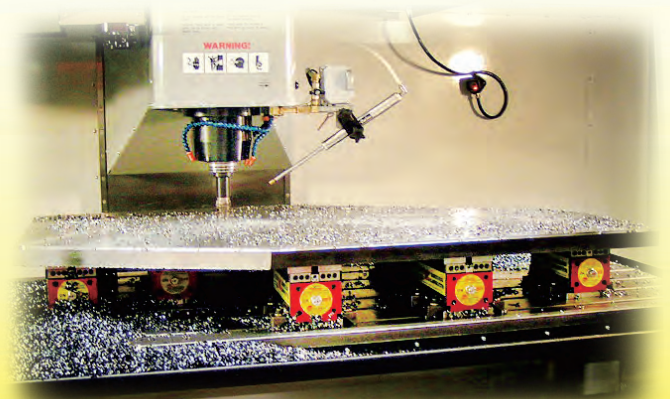
Permanent Magnetic Clamping Block ECB Series
