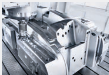
Pre-finishing of a bumper mould Complete machining on a DMU 340 P
