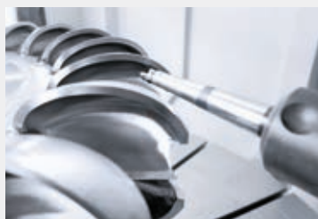
Finishing of a Pelton wheel from a single piece – ø 1,600 mm Complete machining on a DMU 210 FD
