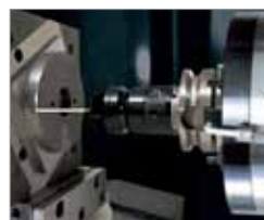
Automatic measuring system
